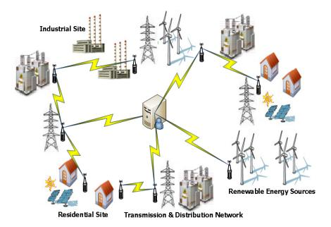
Fig. 1. An illustrative architecture of smart grid using sensor networks. Smart grid can be defined as a modernized electric power T&D network using robust two-way communications, advanced sensors, and distributed computing technologies to improve efficiency, reliability and safety of power delivery and use.
